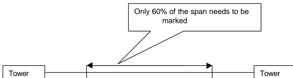
**Figure 5:** Area of span that must be marked
