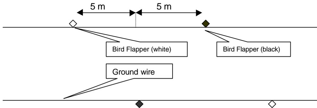
**Figure 4:** Marking method with Bird Flappers on overhead ground wires (viewed from above)
